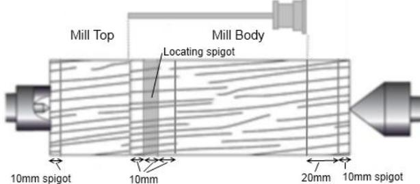
6. Using a parting tool to cut the spigots on each end of the blank down to the size of your chuck (usually around 50mm diameter).
