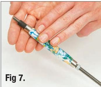
Buff with a cloth until smooth, even finish is achieved. Remove barrel from mandrel. Use instructions provided in pen kit for assembly. Use a Pen Press for best results.
